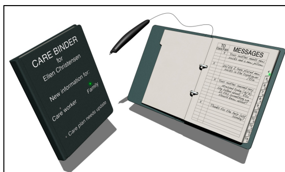
Figure 1. The Augmented Binder employs a pen for the digital capture of messages, and provides notifications of new messages employing RFID technology.
