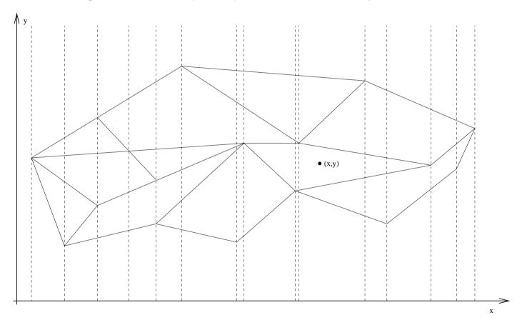
Each dashed vertical line can be represented by a snapshot of a dictionary. Much faster than using copies.
