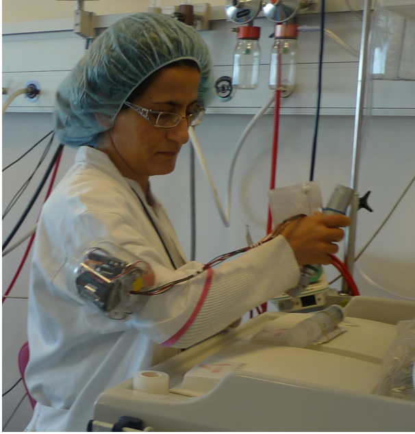
Figure 5. The anesthesia nurse preparing instruments at the anesthesia table. All instruments are tagged with RFID tags and the table has a built-in RFID reader. Moreover, the nurse carries a palm-based RFID reader that reads which instruments she is holding.
