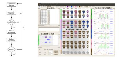
**Fig. 1.** Left: flow diagram for generating SPs with AngelStow. Right: screen shot of AngelStow stowing a vessel calling 5 ports. Labels indicate load list of containers and status of the ballast tanks for the current call, and multi-port vessel view of 5 different calls (current call highlighted) with their corresponding stresses graphs.
