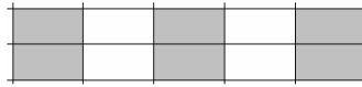
Figure 3.8: Several separate rectangular cell areas that can be described by a single FAP set pr. dimension
